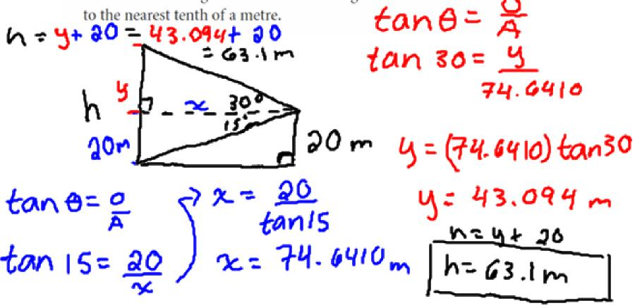
2. A surveyor stands at a window on the 9th floor of an office tower. He uses a clinometer to measure the angles of elevation and depression of the top and the base of a taller building. The surveyor sketches this plan of his measurements.
