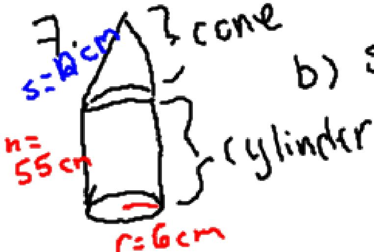
$$b) SA_{ROCKET} = \overbrace{\pi rs}^{\text{cone}} + \overbrace{\pi r^2 + 2\pi rh}^{\text{cyl. or body}}$$
